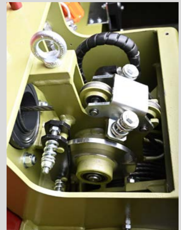
Cable intake brake with cable dispenser
