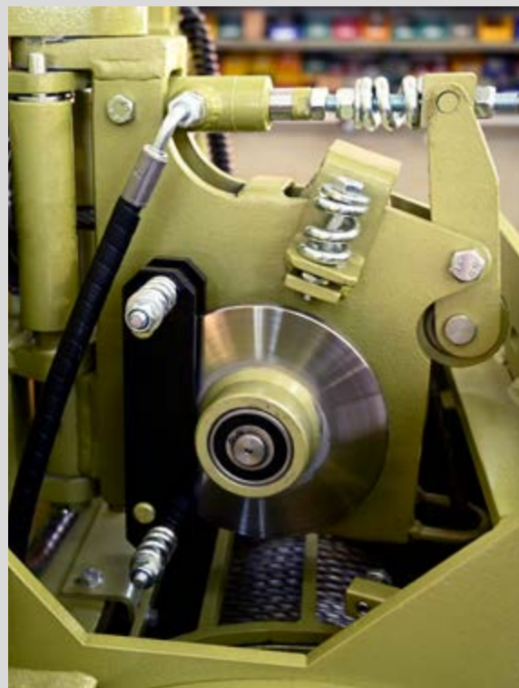
■ Cable intake brake with cable dispenser
